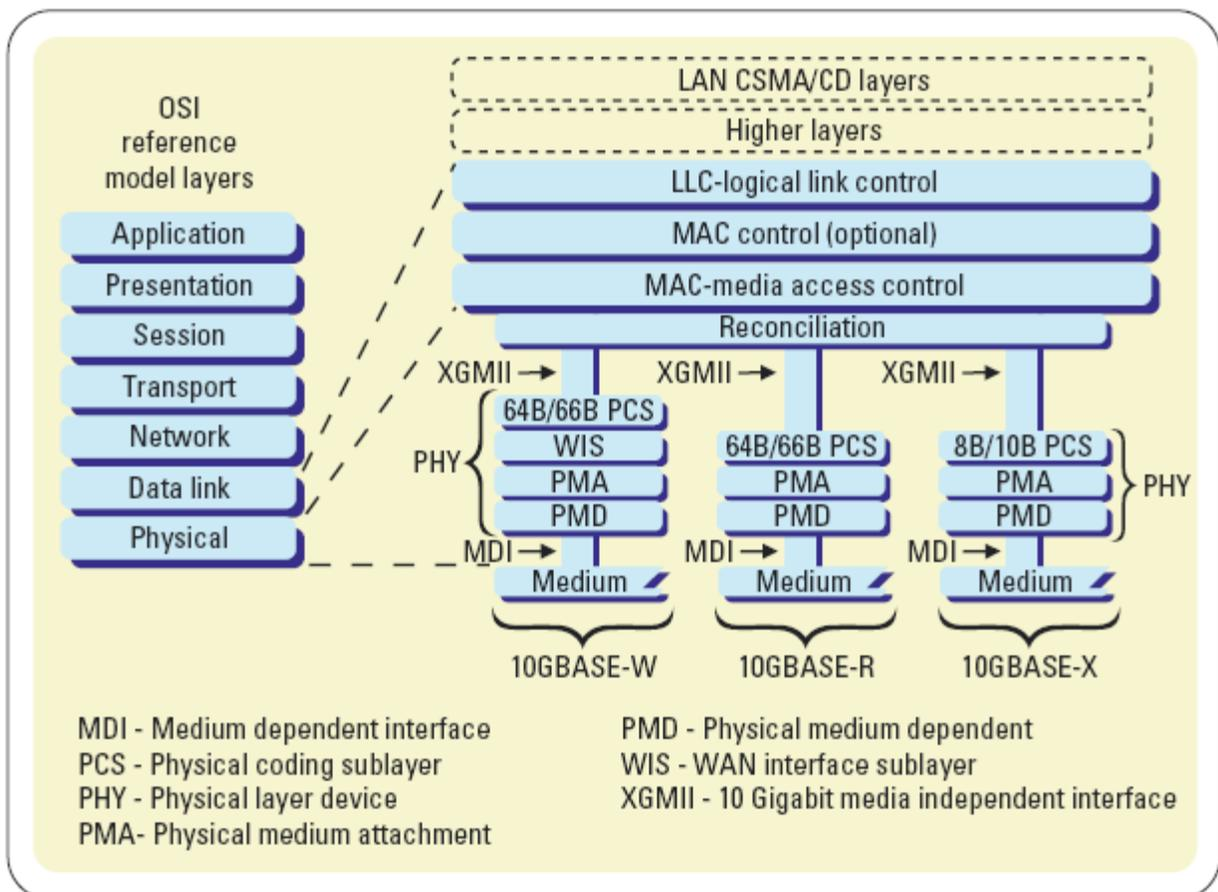
**MDI (Media Dependent Interface)** - the component of the media attachment unit (MAU) that provides the physical and electrical connection to the cabling medium. An MDIX (for MDI crossover) is a version of MDI that enables connection between like devices. MDI ports connect to MDIX ports via straight-through twisted pair cabling; both MDI-to-MDI and
