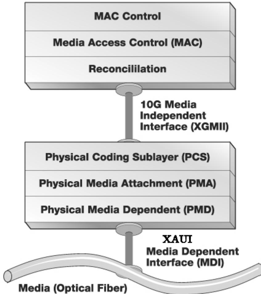
Ethernet is fundamentally a Layer 2 protocol. An Ethernet PHYSical layer device (PHY), which corresponds to Layer 1 of the OSI model, connects the media (optical or copper) to the MAC layer, which corresponds to OSI Layer 2.
