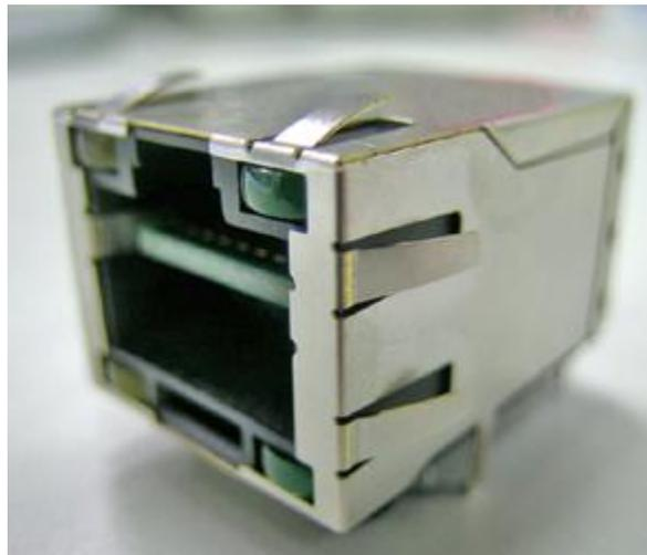
UltraJax provides a high density contact capability with a standard RJ connector. Contact assemblies are housed in both the top and the bottom of the Ultrajax RJ Connector. Now, one RJ connector becomes capable of performing the functions of two connectors. Ultrajax is the first major innovation in RJ connectivity. Pictured above is an UltraJax designed to be built into products attaching to printed circuit boards. In the
