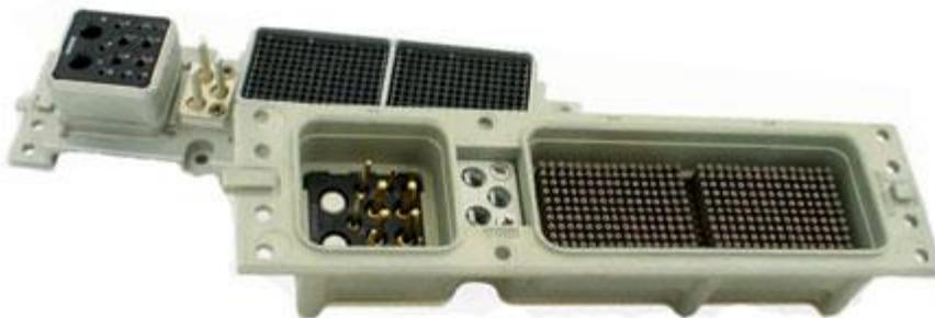
ARINC 600, Rack & Panel connector Series, feature rear release/rear removable low insertion force contacts. The ARINC 600 connectors are available both in environmental resistant and non-resistant versions. The connectors are available in 3 sizes: size 1 (low profile) and size 2 with 3 gangs only while size 3 comprises 6 gangs (the maximum number of contacts of # 22 is 800).
